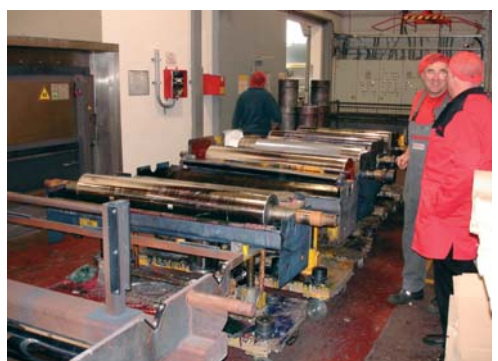
Right: In the preparation room, gravure cylinders with ink residues stand directly in front of the cylinder washing machine.
