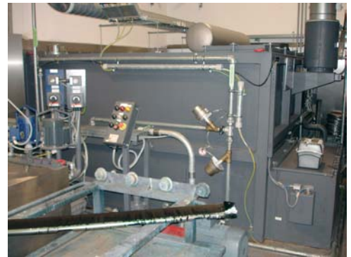
Left: The door of the cylinder washing machine, which is located outside the hazard area, is locked during washing.
