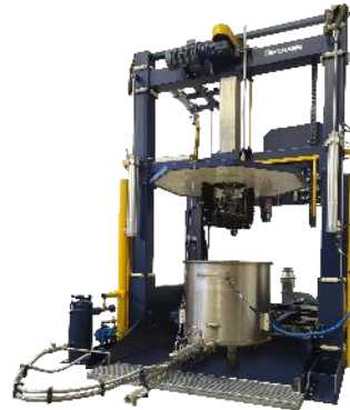
Cleaning systems for mixing vessels and transport containers
